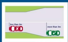
At least 3 metres must be left between your vehicle and the centre dividing line to allow other vehicles to pass safely and not obstruct traffic.
